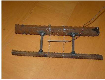
Fig 10: the Strain Gauges with the protection to keep it safe while casting
